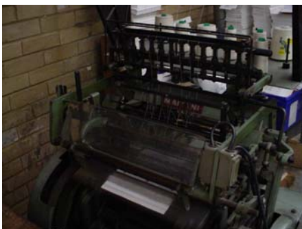
Martini section sewer
